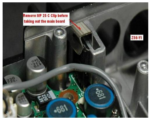
Unclip the spring clip situated at the back mid right hand side of the radio
