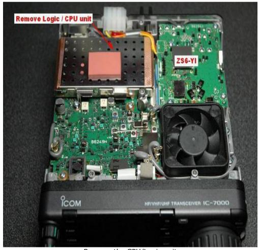
Remove the CPU/Logic unit
