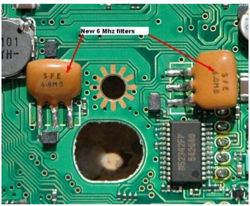
New 6 MHz Ceramic Trap Filters
