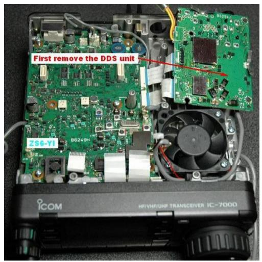
Remove the DDR unit first then the main board
